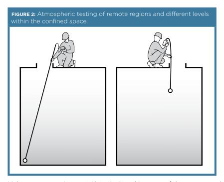
Lighter gases may be vented into the breathing zone of the person conducting the tests. Some gases may be dissolved in liquids and released when the liquid is disturbed or a crust over the liquid is broken and it may therefore be necessary to agitate liquids before monitoring.
