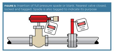
Closing, locking and tagging at least two valves in the piping leading to the confined space (see Figure 6). A drain or vent valve between the two closed valves should be locked open to atmosphere as part of this method.
